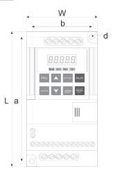
Dimensions of the inverter and location of the measurement holes
